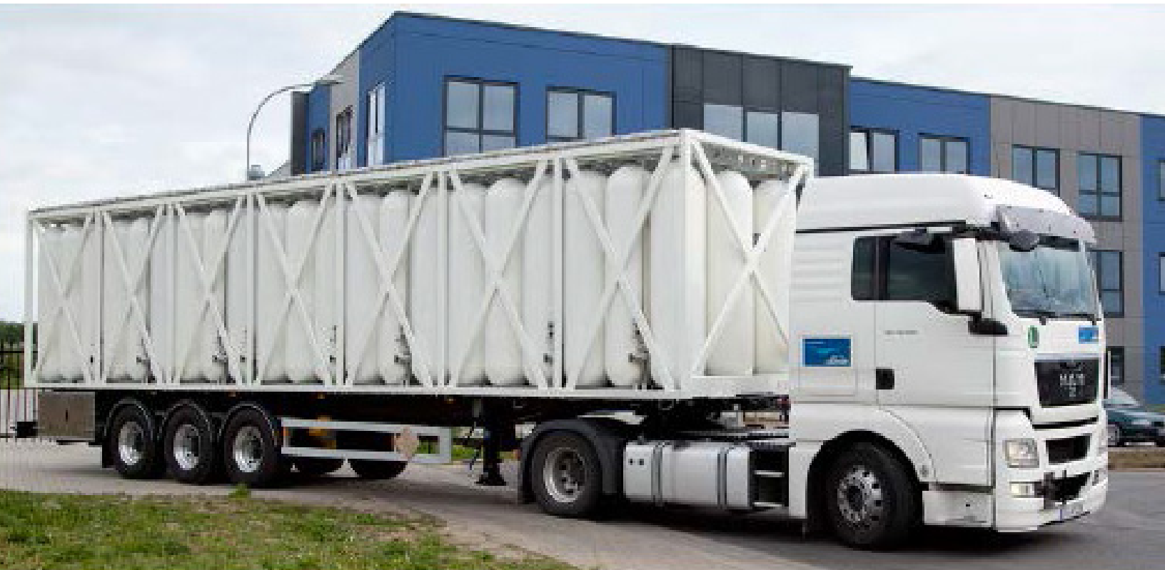
Figure 8: Linde 500 bar trailer with 1,100 kg of hydrogen capacity
