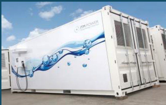
Figure 12: ITM Power's HFuel Unit Generates Hydrogen Gas From Water By Electrolysis
