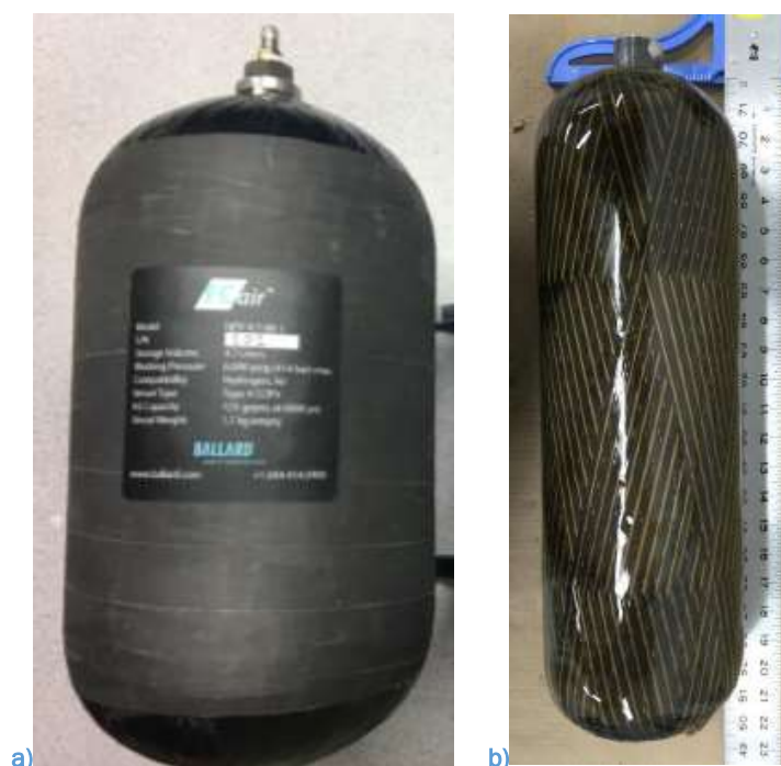
Figure 1. a) 4.7 L and b) 9 L Type IV compressed H 2 COPVs.
